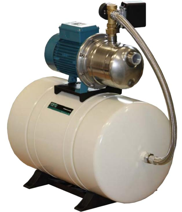
NGXM5-16 jet pump with mechanical switch and 80 litre pressure tank with axial diffuser for reduced noise
